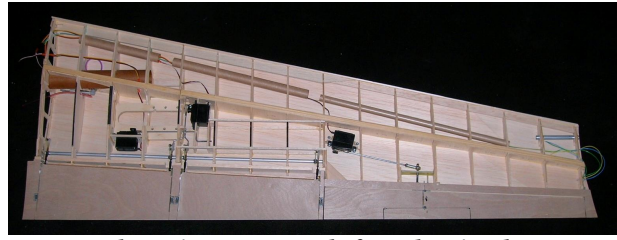
complete wing structure before sheeting bottom
