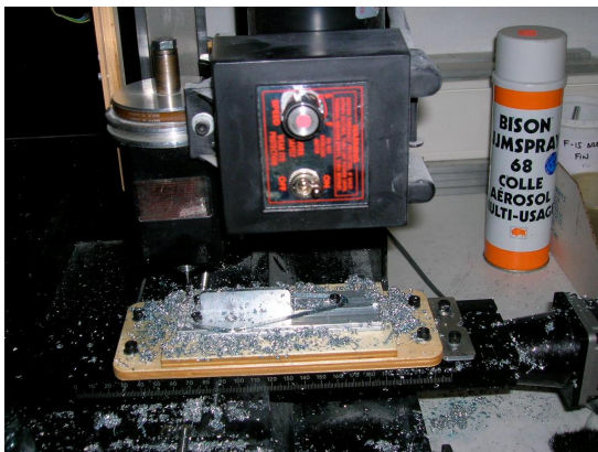
milling a nose retract frame
