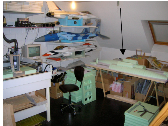
3 D machined sections joined on aluminium spar
