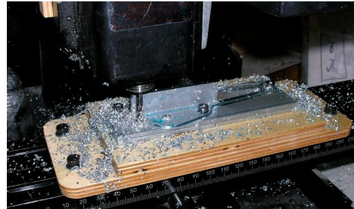
milling the main gear retract frames
