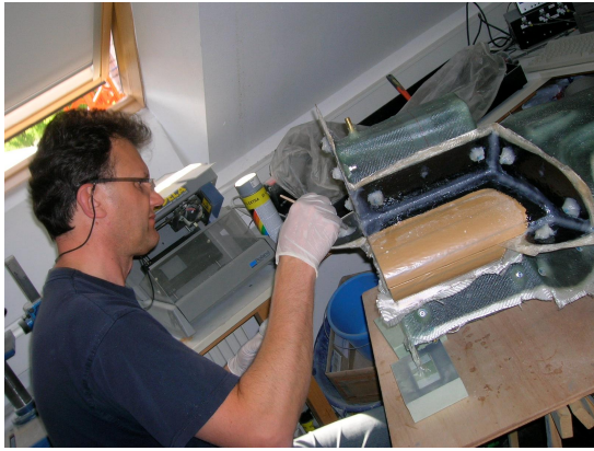
laying up the moulds of the fuselage...
