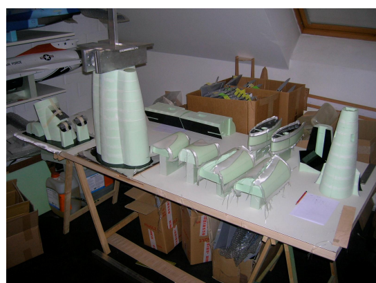
fibreglassing the foam parts
