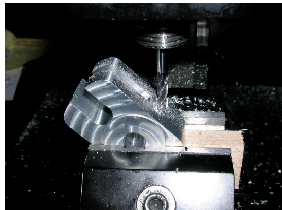
machining work on the main retract pivot block
