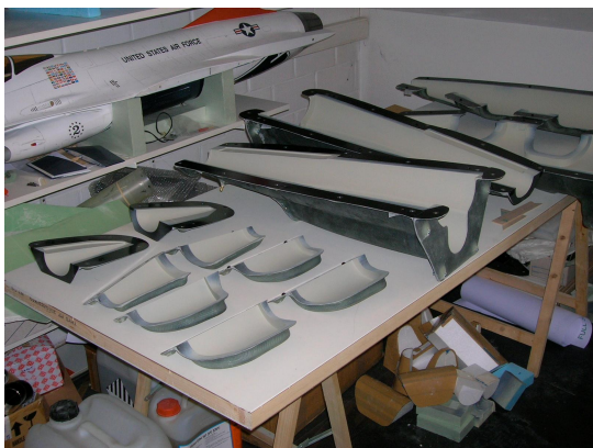
primer sprayed into the moulds
