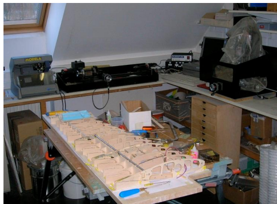
wing structure on foreground, CNC machines from left to right: a Roland Modela, a Sherline CNC lathe and a Sherline CNC mill
