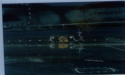
Original photograph of actual subject aircraft showing inspection cover of the location for positioning ground lifting equipment.
