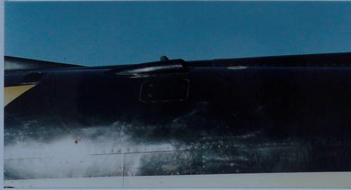
Original photograph of actual subject aircraft showing cooling air scoop on top of fuselage (present paint scheme).
