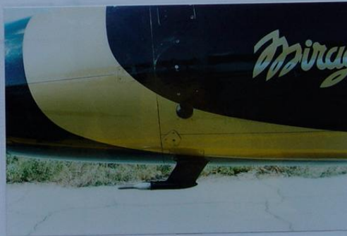
Original photograph of actual subject aircraft (present paint scheme) showing the opening above the TAT probe on the left side of forward fuselage.
