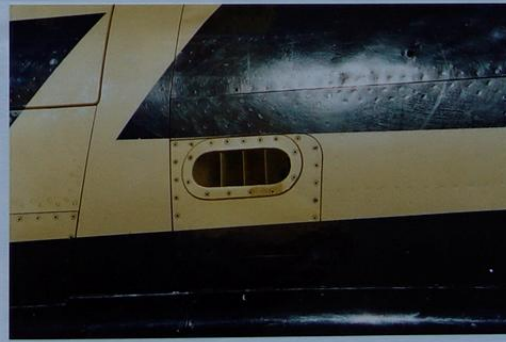
Original photograph of actual subject aircraft showing bleed air vent on right side of fuselage (present paint scheme).
